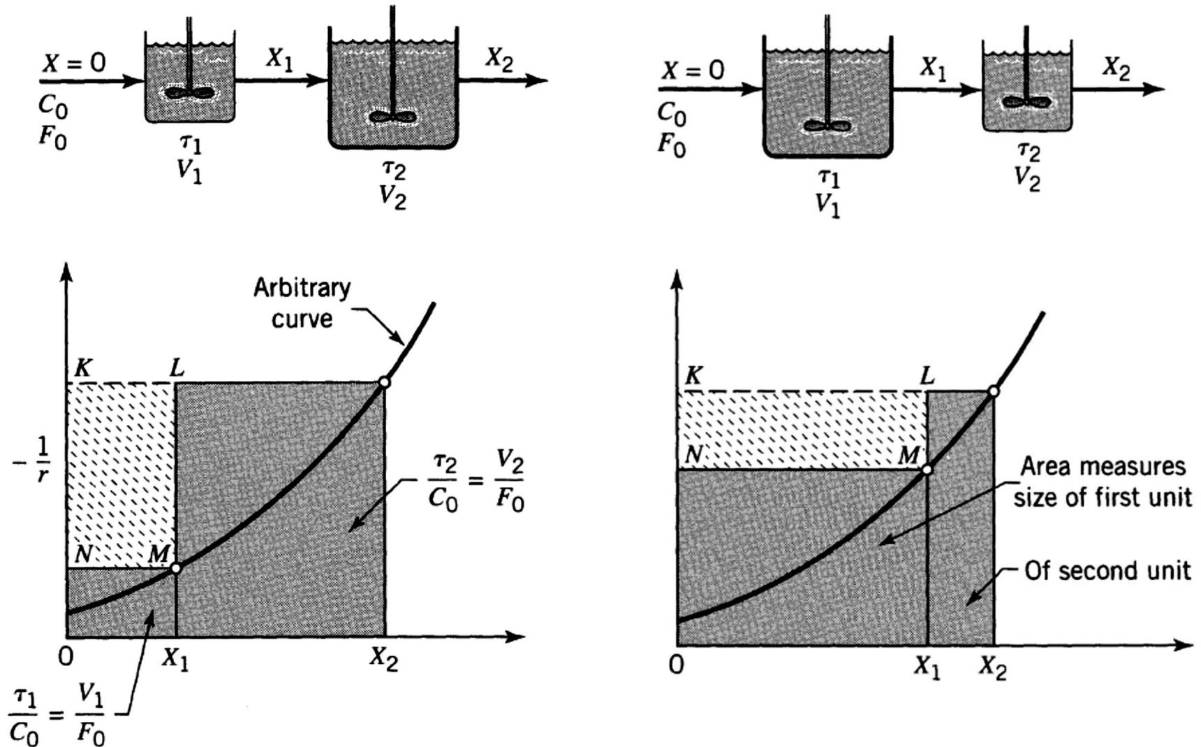
**Figure 4-8** Graphical representation of the variables for two mixed flow reactors in series.
