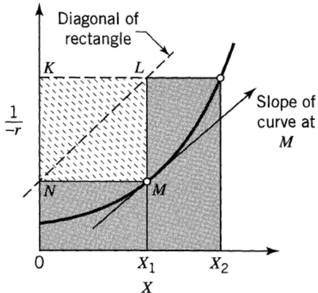
**Figure 4-9** Maximization of rectangles applied to find the optimum intermediate conversion and optimum sizes of two mixed flow reactors in series.
