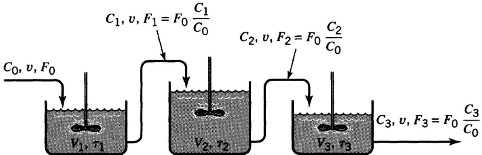
**Figure 4-6** Notation for a series of unequal-size mixed flow reactors
