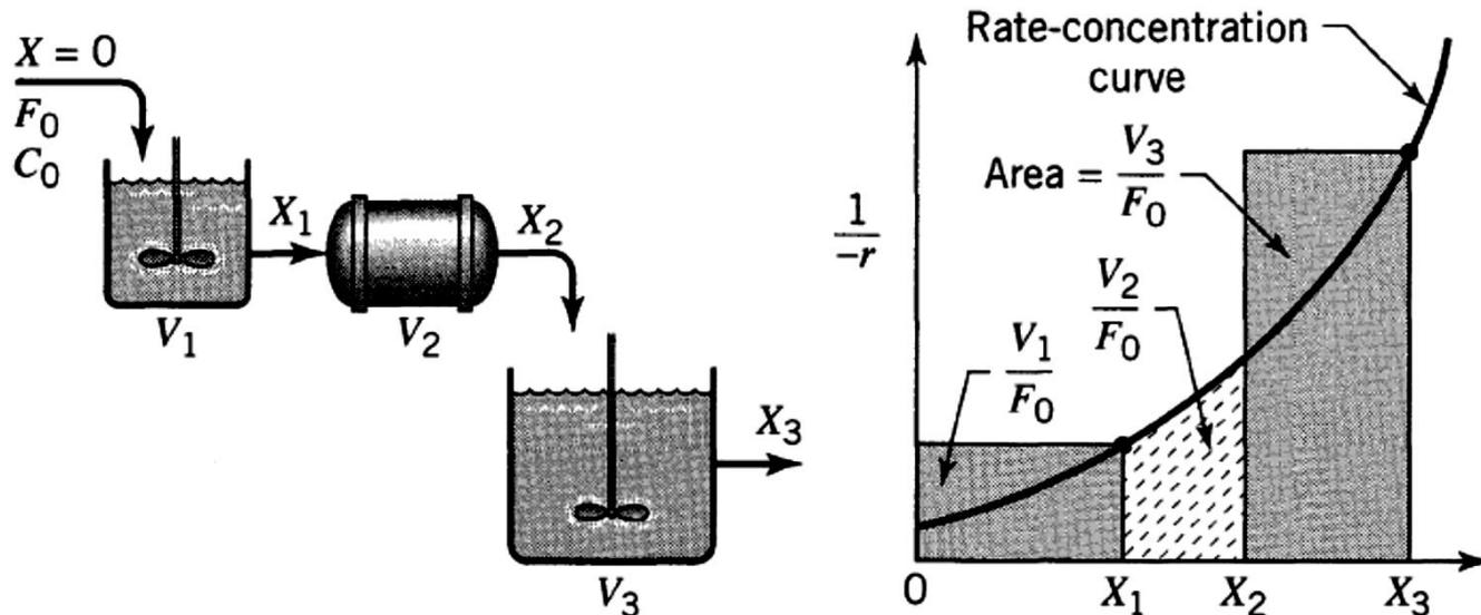
**Figure 4-10** Graphical design procedure for reactors in series.
