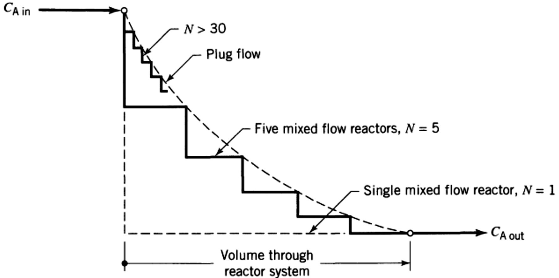
**Figure 4-3** Concentration profile through an  $N$ -stage MFR system compared with single flow reactors.
