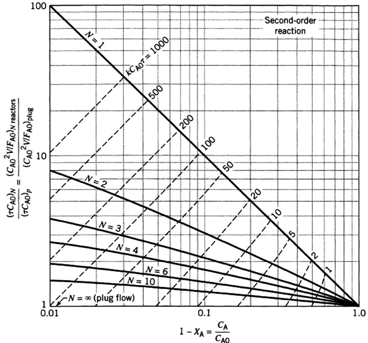
Fig.4-5: Comparison of performance of a series of  $N$  equal-sized MFRs with a PFR for the 2<sup>nd</sup> order reactions with negligible expansion
